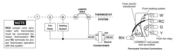
Figure 5. Typical Wiring Diagram for Heat Only, 3-Wire, Single Transformer Systems
